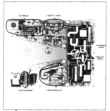
Photo  $C^{\mathbb{P}}$ . A close-up of the RF circuit board after the plastic cover has been removed.
