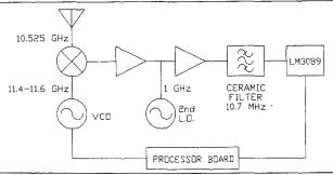
Figure 2. Block diagram of the radar detector.
