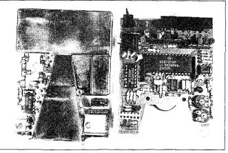
Photo B. Inside the radar detector. RF board on the left. Controller board (not used) on the right.
