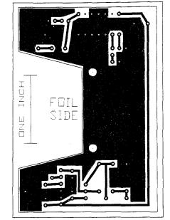
Figure 6. Foil side of the PCB.
